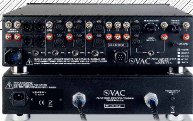
ABOVE: Outboard PSU [bottom] includes an extra transformer and umbilical to feed the optional MM/MC phono board included in our Master Preamp [top, right]. Six line inputs are available, inc. one direct (HT) and three with balanced (XLR) options. Dual preamp outputs are offered on RCAs and balanced XLRs
