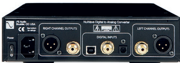
ABOVE: The rear panel plays host to coaxial, optical and USB digital inputs in addition to balanced (XLR) and unbalanced (RCA) analogue outputs
